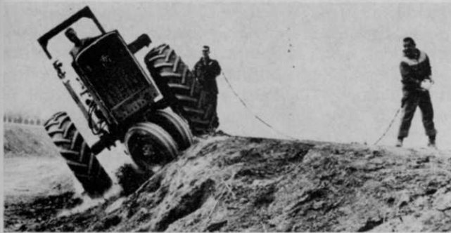
Tractor reaches speed and incline which starts rollover.
