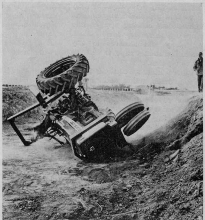
Protective frame in this test protects dummy, but in regular operation would likely prevent serious injury or death to operator.
