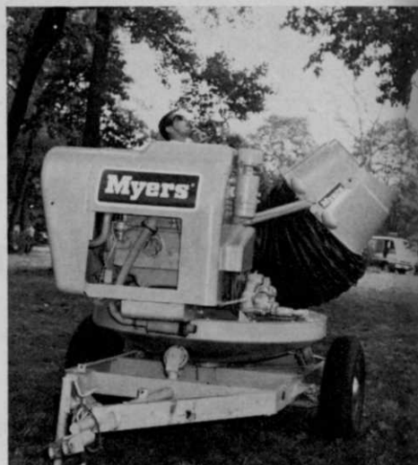
Myers demonstrated new TT29 Tall Tree mist sprayer. Equipment according to Myers representative is designed especially for tree protection, mosquito control, leaf windrowing, brush burning and sanitation spraying.
