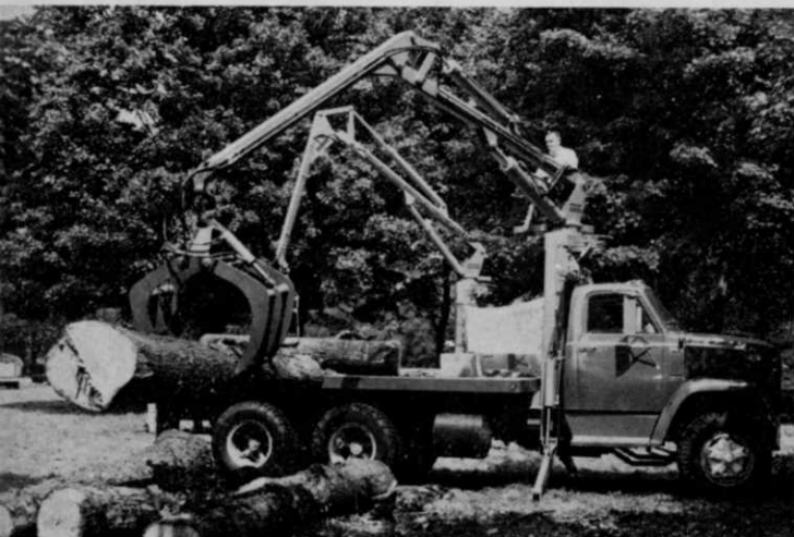
Prentice Hydraulics, Inc., Prentice, Wis., showed their hydraulic loaders, left, for logging and other tree service company utilization.
