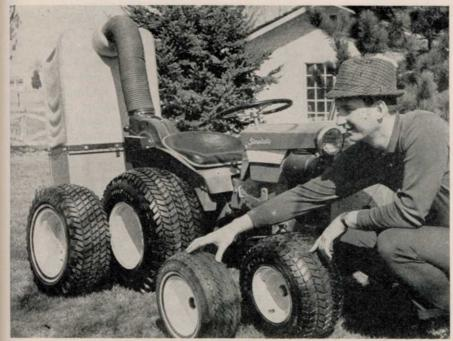
Terra-Tire by Goodyear has been so designed that combined weight of man and tractor exerts less pressure than if the man were on foot. Walking pressure is about 24 pounds per square inch, 2 to 3 times more than if he were riding on a Terra-Tire-shod garden tractor. Tires also enable tractor to ride through mud, sand, and snow where tractor with conventional tires might bog down. For data, write Goodyear, Akron, Ohio 44316.
