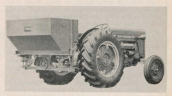
Piggyback Broad-Caster, Model 413-3, engineered for rough terrain. Gives excellent pattern on level ground. A 15 cubic foot capacity hopper, using twin fans to insure an even spread pattern. Unique single belt drive system eliminates gear boxes, chains, and troublesome drives. Application rates from 25 to 400 pounds per acre. Write: L. L. Larson Machine, Inc., Princeville, Ill. 61559.
