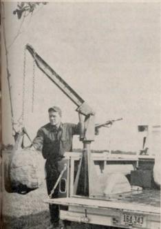
Hydraulic truckcrane designed for one-man loading and unloading. Hydraulic jack is heart of lifting mechanism. Features 360-degree rotation, and can be mounted on any style truck body or on loading dock. Replaces forklift for many jobs when mounted on floor dolly. Two sizes, 1500-lb. and 2500-lb. Source: Ideal Crane, Bert Parkhurst and Co., 15051 E. Admiral Place, Tulsa, Okla.
