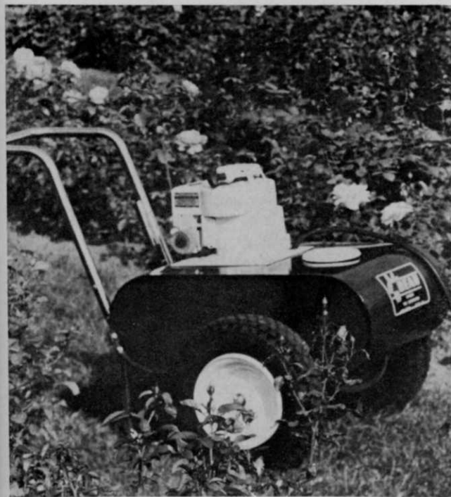
Self-contained power sprayer with 10- or 20-gallon porcelainized steel tank, above, from John Bean. For weeds, pests and mosquito-infested areas. Trojan sprays 3 gallons per minute at 60 pounds pressure. Self-lubricating, fiberglass pump, located inside tank, has only one moving part. Jet agitation and constant spray pattern. Catalog, S-03, John Bean Div., Tipton, Ind.
