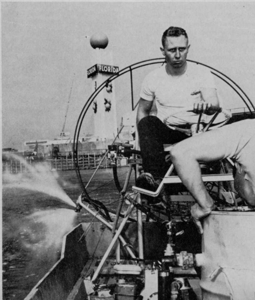
Lakes within exhibition area of recent New York World's Fair were subject to extensive growth of weeds and algae. Sheridan turned to air boats to avoid turbulence in shallow lakes. Copper sulfate was ejected to rear and on both sides of propeller. Spray covered almost 60 feet on each side of unit.
