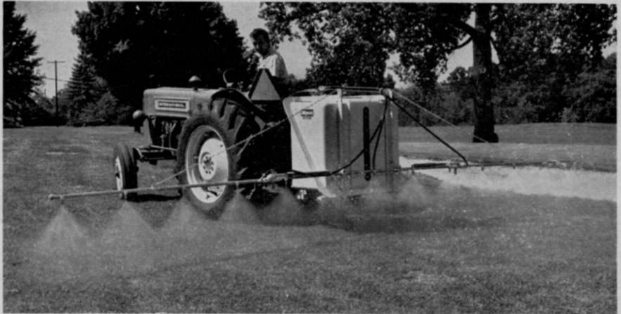
100TM - Tractor-Mounted, 100 Gallon, PTO Sprayer
