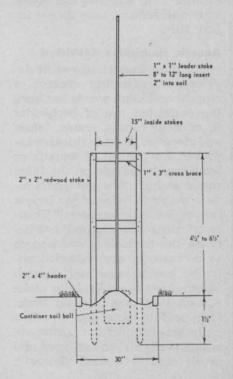
stake meets the conditions of only 4 and 5. The 2-in.-square stake generally fails in requirements 2,3,4, and 6. The 2-in. by 4-in. stake, or 4-in.-square stake, generally fails in all requirements but 1. The double or triple 2-in.-square stake is an improvement, but fails to meet condition 6, and partially fails in 2 unless the tree is specially secured with loop wire ties.
