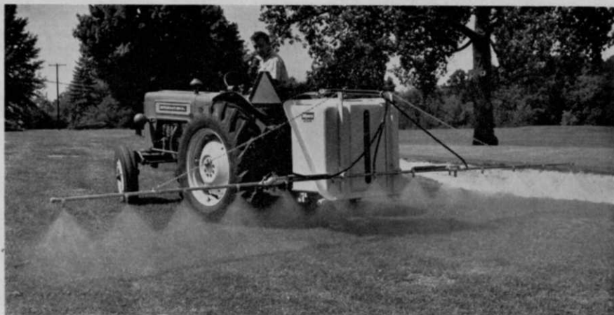
100TM - Tractor-Mounted, 100 Gallon, PTO Sprayer
