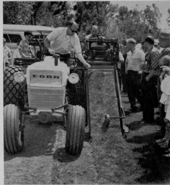
Nunes Sod Harvester was demonstrated by John Nunes of Cal-Turf Farms. Nunes reported unit will lift, roll, and palletize up to 1200 square yards per hour.
