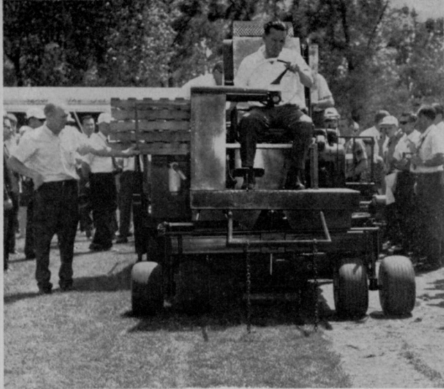
Princeton Turf Farms' Sod Harvester is capable of handling up to 10,000 square feet of cut and palletized sod per hour, based on report during field day demonstration. Wiley Miner, president of Princeton Turf Farms, on hand for the field day, was instrumental in development of the machine which operates with 3 men and produces uniform pads of folded sod, stacked on pallets.
