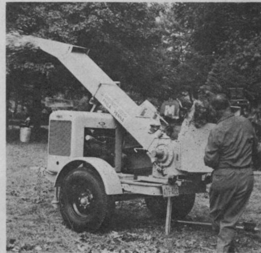
Pitman chipper built by Pitman Manufacturing Co., Grandview, Mo., features according to the maker, shallow cutting action, unique self-aligning cutting blade and emergency safety brake.
