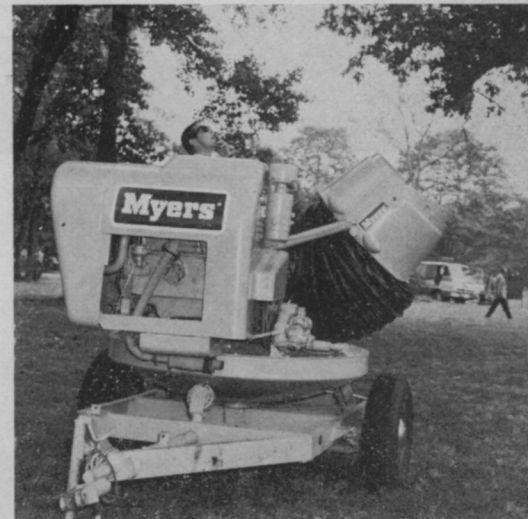
Myers demonstrated new TT29 Tall Tree mist sprayer. Equipment according to Myers representative is designed especially for tree protection, mosquito control, leaf windrowing, brush burning and sanitation spraying.
