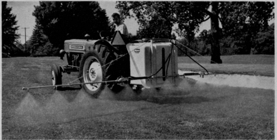
100TM - Tractor-Mounted, 100 Gallon, PTO Sprayer
