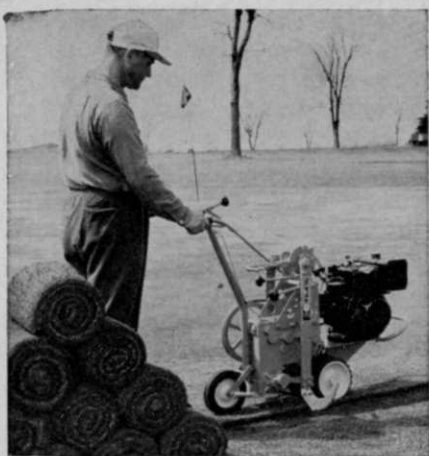
Ryan Jr. Sod Cutter works fast. Cuts sod clean and even, 12" wide, up to 2½" thick.
