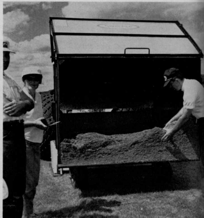
Rogers Turf Sweeper was demonstrated by Clarke H. Staples, right. Unit has 5-foot sweeping width with 5-cubic yard hopper, also is equipped with thatcher-thinner attachment.
