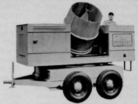
MODEL 303T ROTOMIST biggest performer among mist-type shade tree sprayers. 40" fan, 60,000 CFM air volume.
