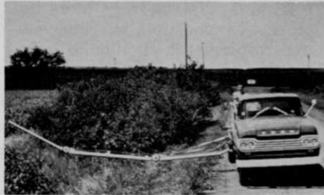
ROTOCAST® specially designed for roadside weed control. Teardrop discharge head provides reach plus close-in coverage.
