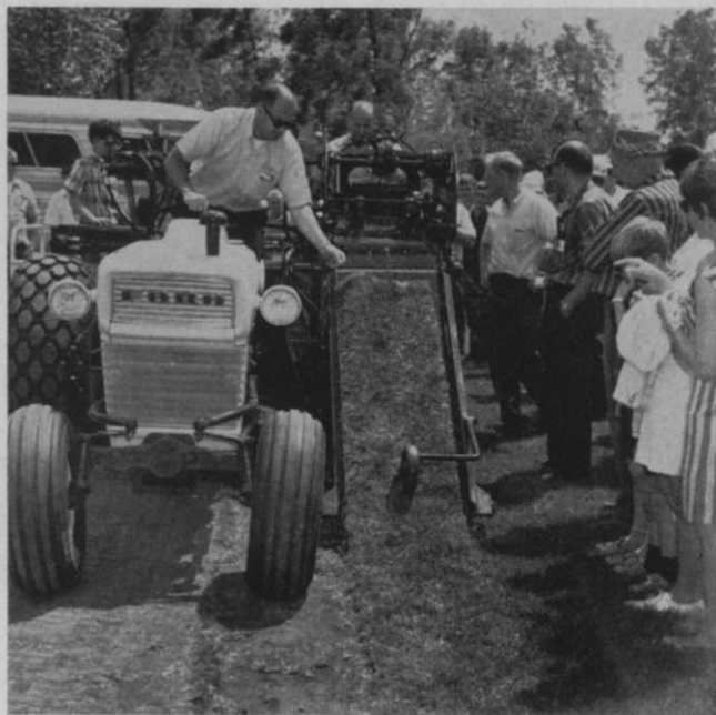
Hadfield Sod Roller , designed to fit on Ryan sod cutter, was among new equipment demonstrated. Hadfield reports unit operates strictly as 1-man operation and is particularly well adapted to smaller sod farm. Roller is manufactured by Hadfield at Oxford, Mich.
