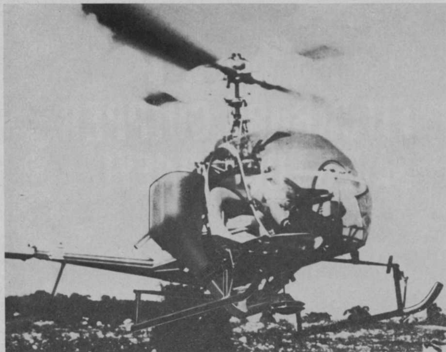
Uniform granular herbicide or fertilizer application is said possible with the Evergreen spreader introduced by Evergreen Helicopters Inc., McMinnville, Oregon.
