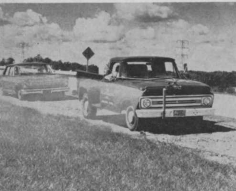
Multi-Purpose Myers Industrial Sprayer is designed for mounting on pickup. Remote control nozzle is optional.
