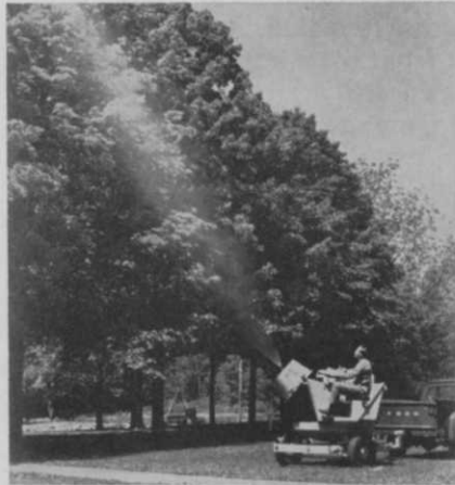
Tall Tree Mist Sprayer , shown here in action, delivers 30,000 cfm air volume. Entire Myers unit swivels through 360°.
