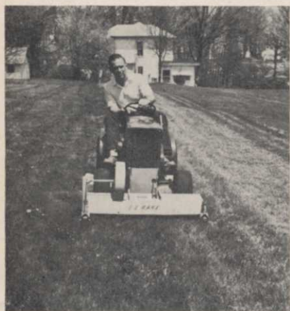
Thatch removal was part of the bluegrass test; here performed with an attachment to the John Deere garden tractor.
