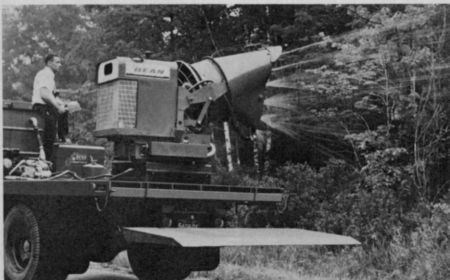
Broadcast pattern spray head introduced by John Bean, is shown here operating from hand-held remote controls. The attachment, called "Rotocast," is powered by a 4-cylinder, air-cooled engine, and can discharge 10 to 40 gals. of spray per minute at 40 p.s.i. Remote controls rotate the sprayer 210 degrees horizontally. Air stream is adjustable through an arc 45 degrees downwards and upwards. More complete specifications can be obtained by writing for Catalog L-1496, to John Bean Division, Box 9490, Lansing, Mich.
