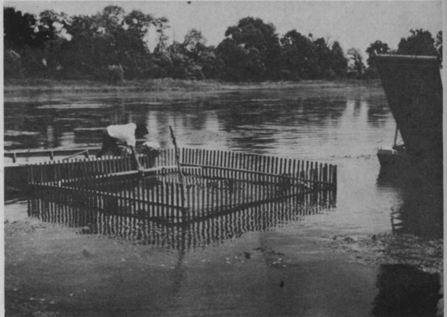
"Bottomless pit" proved the solution to disposing of the harvest. Disposal bin of snow fence tacked to a 12 ft. square frame rides with the tides and has an almost limitless capacity. Cut, trapped weeds rot in two to three weeks, then bin is removed.
