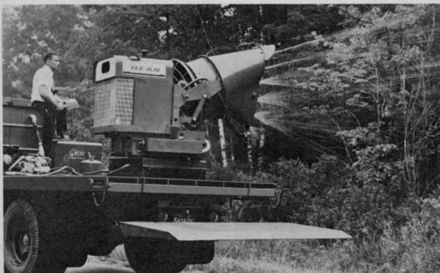
Broadcast pattern spray head introduced by John Bean, is shown here operating from hand-held remote controls. The attachment, called "Rotocast," is powered by a 4-cylinder, air-cooled engine, and can discharge 10 to 40 gals. of spray per minute at 40 p.s.i. Remote controls rotate the sprayer 210 degrees horizontally. Air stream is adjustable through an arc 45 degrees downwards and upwards. More complete specifications can be obtained by writing for Catalog L-1496, to John Bean Division, Box 9490, Lansing, Mich.
