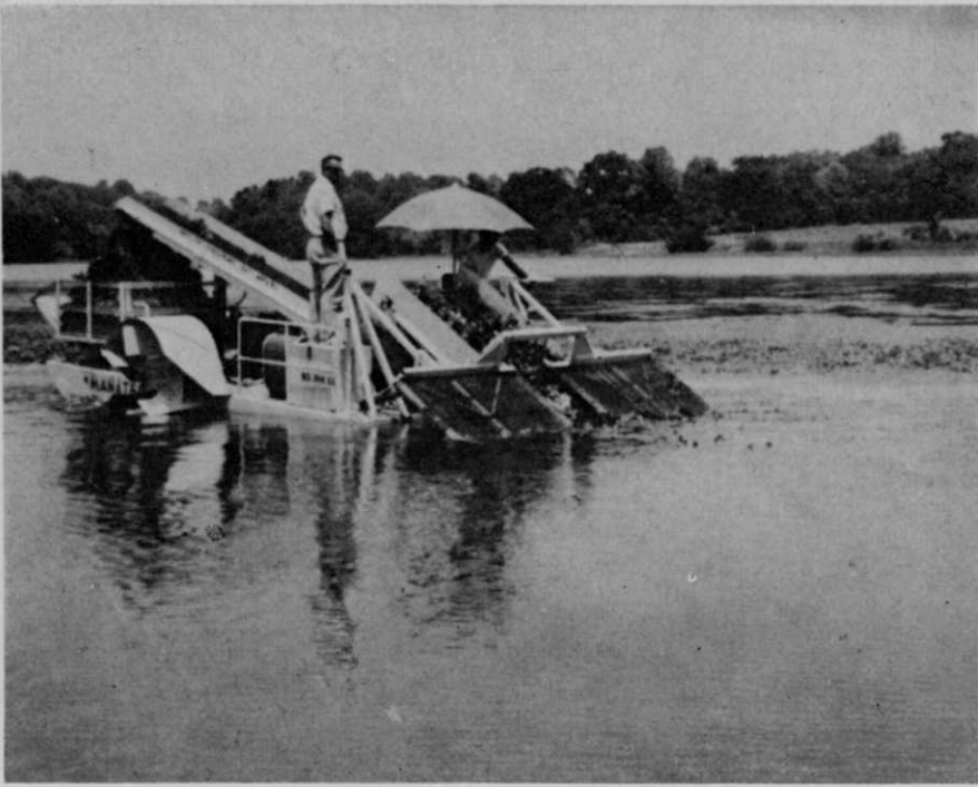
"Manatee", underwater weed cutter, clips waterchestnut 8 in. below water surface. Conveyors dump harvest into a large basket that holds over 100 cu. ft. of the water weed.
