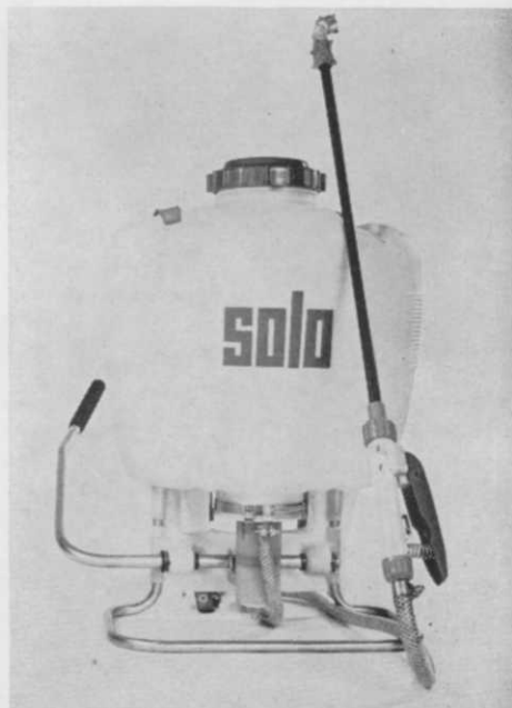
SOLO KNAPSACK HAND SPRAYER 425 Capacity, 4 gallons. "Lightweight" weighs 8 lbs. Delivers up to 16 feet in height.
