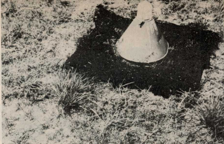
Standard type MC-1 cutback asphalt used in Texas A&M study gives a thin film which barely covers the soil surface.
