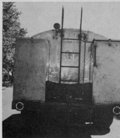
Two 60-gal. stainless steel tanks, mounted behind 2000 gal. water tank, are shown in this rear view of, all-purpose vegetation maintenance spray rig described in this article.
