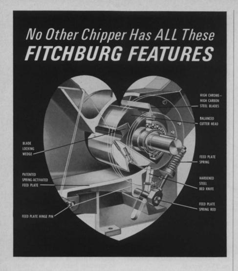
Look inside a Fitchburg Chipper—note its heart—the spring-activated feed plate. No other chipper has this patented feature that adjusts to the size of the wood up to the machine's rated capacity. Chipping is smoother, quieter, faster, permitting the chipping of larger size wood without the need for extra power or the cost of extra fuel.
