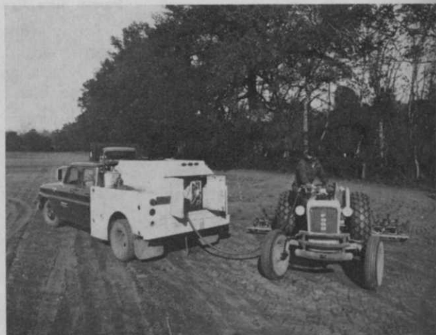
The Farm's Mobile Tanker delivers fuel to field equipment. Many of the Farm's tractors, compressors, etc., are being switched to diesel for higher economy.
