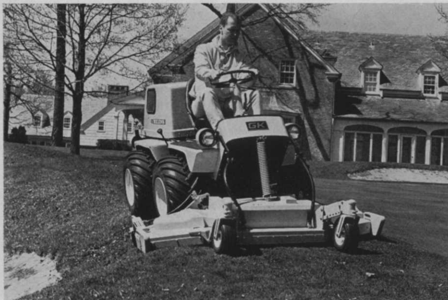
Ground-hugging mower attachment, with 15" wings, enables GK to follow ground contour as on this grass strip between green and sand trap.
