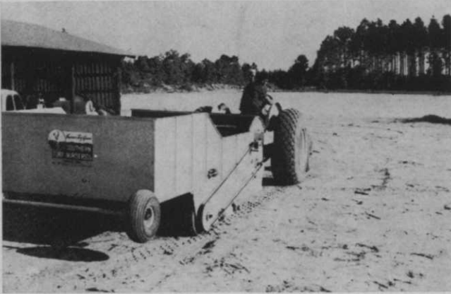
Fully automatic turf planter, used for golf course fairways and other large turf areas, scatter sprigs uniformly and is self-feeding.
