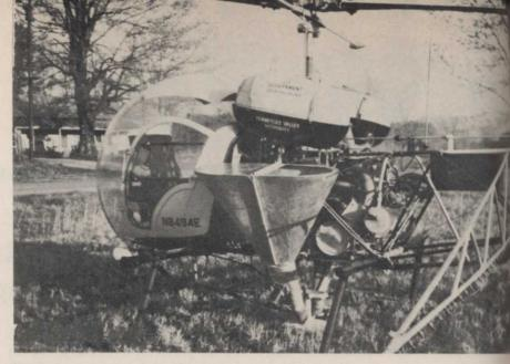
A Bell helicopter (right) is equipped with two 60-gallon bins that tote pelleted material which is fed through chutes to a centrifugal spreader.
