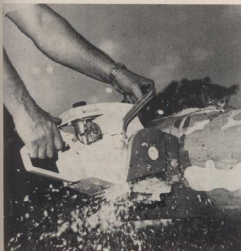
Automatic chain lubrication is one of the improvements added to new Wright chain saw model C-40A. The device is activated from a worm gear with cam, directly from the saw crankshaft. A manual system may be used to override the unit if desired. The saw weighs 16½ lbs., and will take a 14-, 17-, and 21-inch hard nose bar and a 25-inch roller nose bar. For more details contact Wright Saw Div., Thomas Industries, Inc., 207 E. Broadway, Louisville, Ky.
