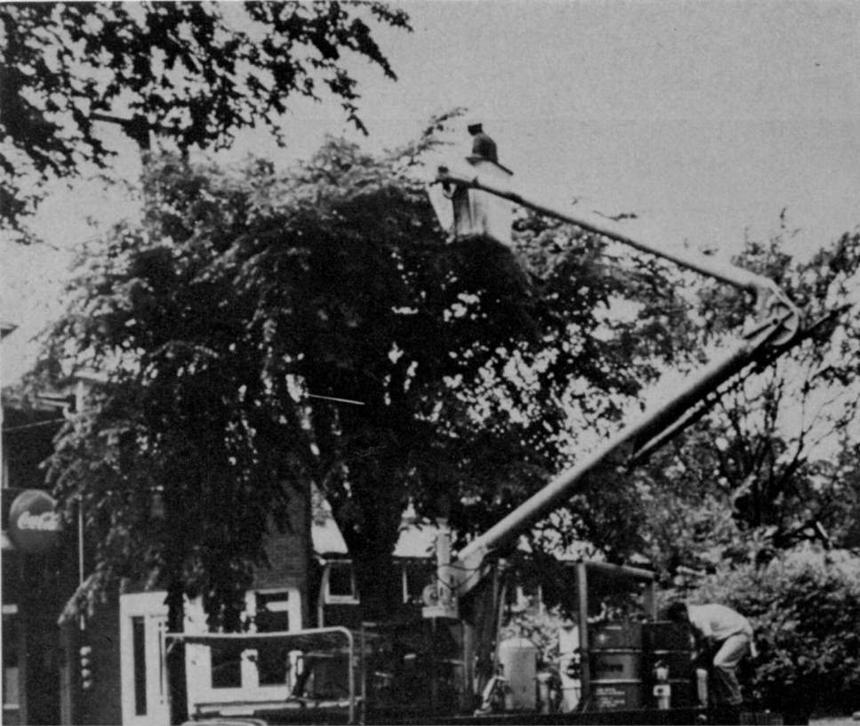
Skyworker was used to apply growth regulator on trees during May in Roanoke, Virginia.
