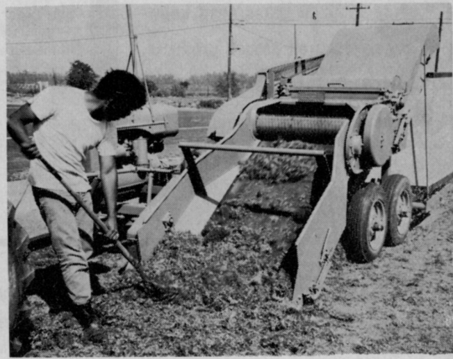
Hybrid bermuda harvester shreds, chops, and screens stolons in one operation; conveys them into bulk bins carried on back of machine.
