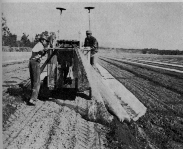
New machine , developed by Tri-Cal Co., fumigation technique specialists, quickly removes sheeting prior to planting; reduces labor costs.
