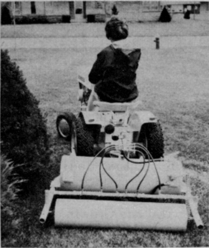
Liquid weed killer drips onto a roller of this Model 101 Commercial 36 inch Pull-Type Drip Roller Unit from Lakes Supply Co. Liquid transfers to ground as the applicator travels. This process eliminates spray drift and allows closer approach to flowers and shrubs, the manufacturer claims. Three models all have adjustable drip rate, filters, and pump gear. Lakes Supply Co., Inc., Dundee, Ill. is the distributor.
