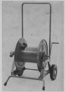
New Hannay portable hose reel handles 60 to 250 ft. of  $\frac{9}{8}$  to 1-in. I.D. hose for liquids or gases up to 300 psi, and temperatures from -20 to +180 degrees Fahrenheit. Rewind is by direct hand crank with an adjustable drag device to brake or lock the reel. The new models are permanently mounted on tubular steel frames. They feature self-aligning front and back bearings. Complete information is available from Clifford B. Hannay & Son, Inc., Westerlo, N. Y. 12193.
