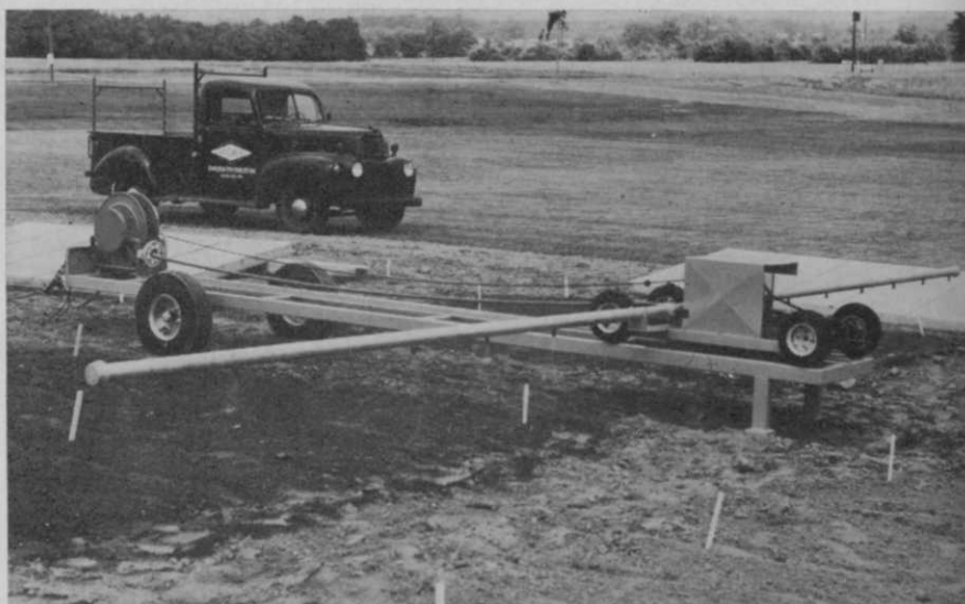
Rainfall to order. Specially constructed mechanical rainmaker, used on a research farm in Ambler, Pa., can deliver any desired amount of "rainfall" simply by setting a timer. Upper part of rainmaker device rolls back and forth on tracks discharging water from 12 sprinkler nozzles mounted on a 22-ft. boom. Entire machine is portable and is wheeled from plot to plot. Primary application is to determine effectiveness of new weedkiller compounds and combinations. To eliminate variables caused by normal rainfall, test plots are covered by a plastic film tent after being saturated by machine-made rain.
