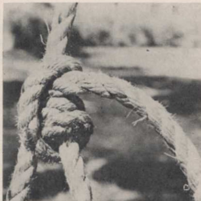
Fig. 2. (below) The sliding hitch knot allows climbers to change their height to any desirable working altitude. It is used just above the saddle snap, well within reach of the tree surgeon.
