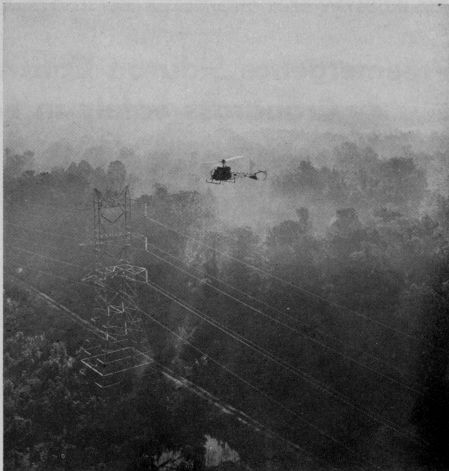
Combined with a particulating agent, Tordon can be used in aerial applications such as this, making it applicable for brush control along hard-to-get-at powerlines in difficult areas.
