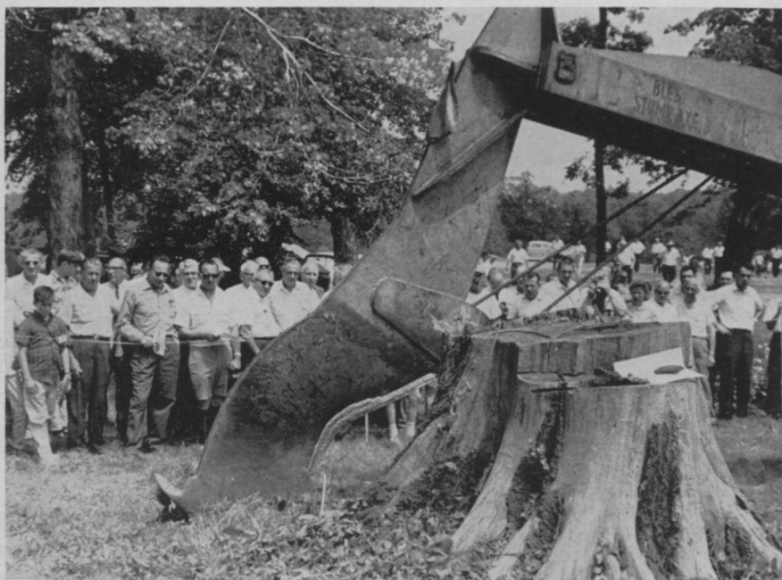
Over 20 suppliers demonstrated their equipment at U.S. National Arboretum for ISTCers. Shown here is a massive stump axe made by Bles Stumpax Co. Arborists watched this unrelenting claw dig out the huge stump in under one hour, a job that would otherwise have taken three men three days to accomplish. Also shown were skylifts, chippers, sprayers, dusters, chain saws, and stump cutters. Shade of trees protected spectators from 98° temperature during the activity.
