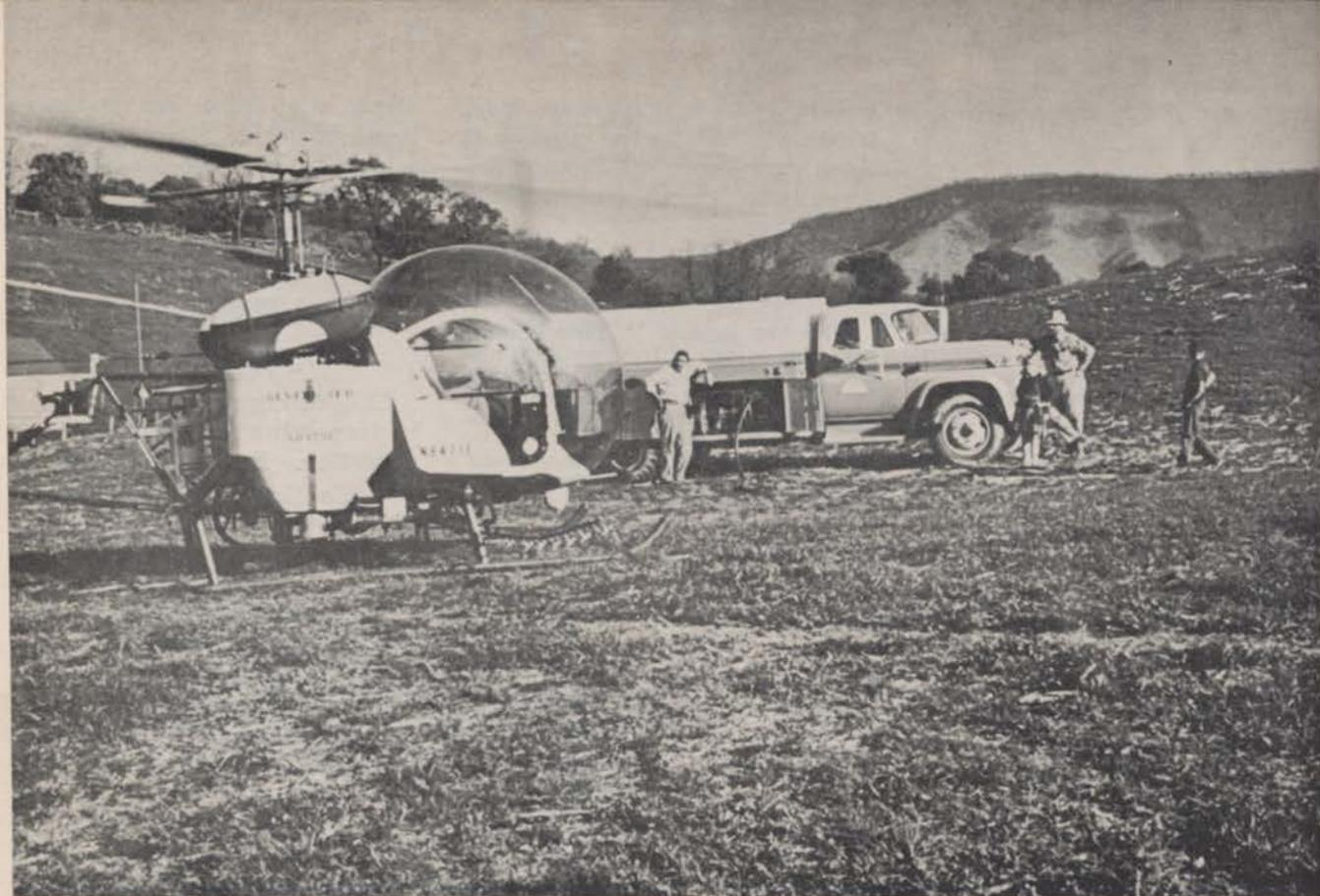
Equipped for pastureland spraying, helicopter tanks are loaded with herbicide from companion service truck.
