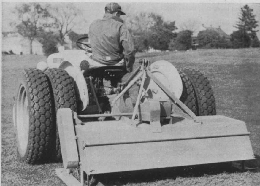
Two sets of soil-engaging blades are principal features of this soil renovator designed for fairway use by West Point Products Corp. Renovating blades are mounted on rotating shaft and are preceded by slicing knives mounted on a stationary shaft performing thorough renovation. Renovating blades can be disengaged to use this equipment as a slicer only.
