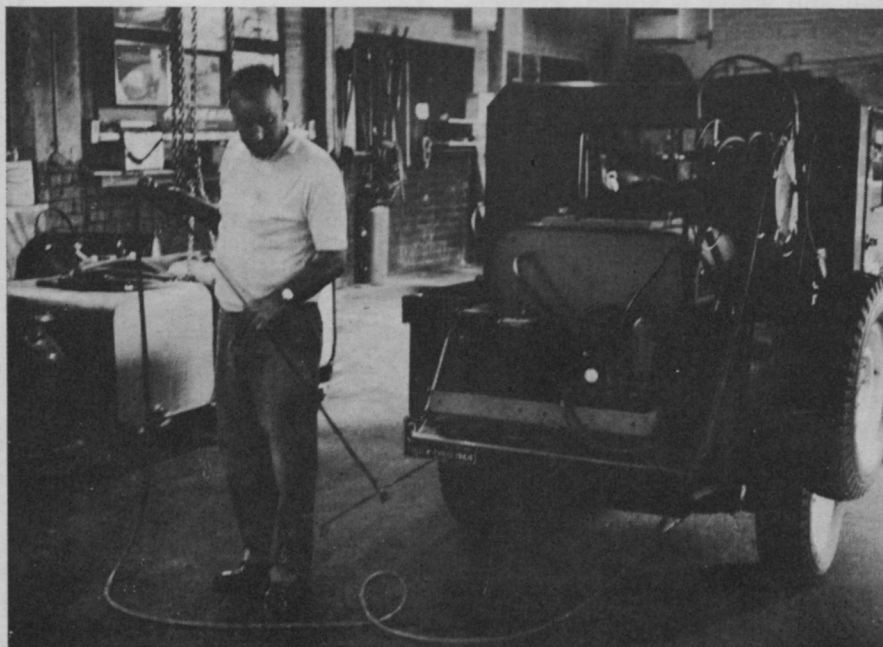
Azo owner, Larry Smith, shows a residential trident spray wand. He explains that some men never learn how to spray a lawn. Jeep-mounted rig is a Hardie Town & Country, 25-gal. sprayer.
