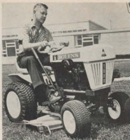
New Bolens Husky 1000 has extrawide tires to protect turf, 6 forward and 2 reverse speeds.
