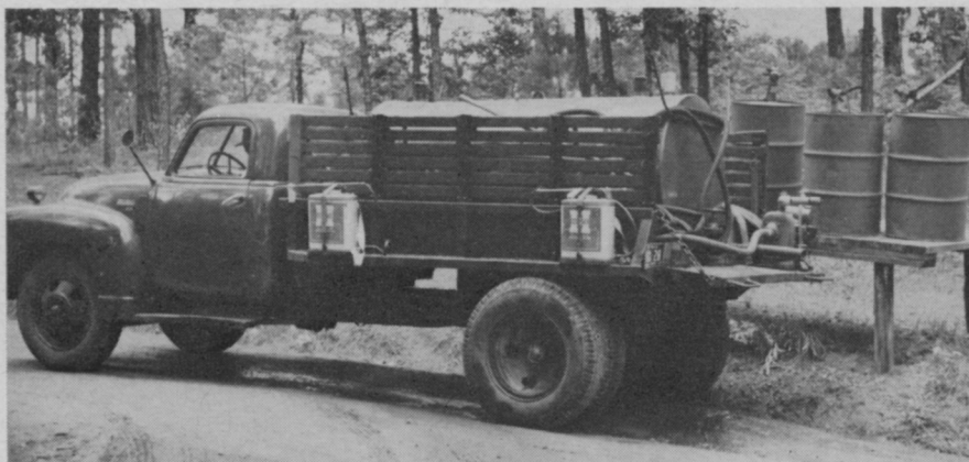
1 1/2-ton truck with 500-gal. tank and small pump for fighting fires, if needed. In winter, Collaway Gardens keeps several 50-gal. drums on hand for similar use with pickup trucks.
