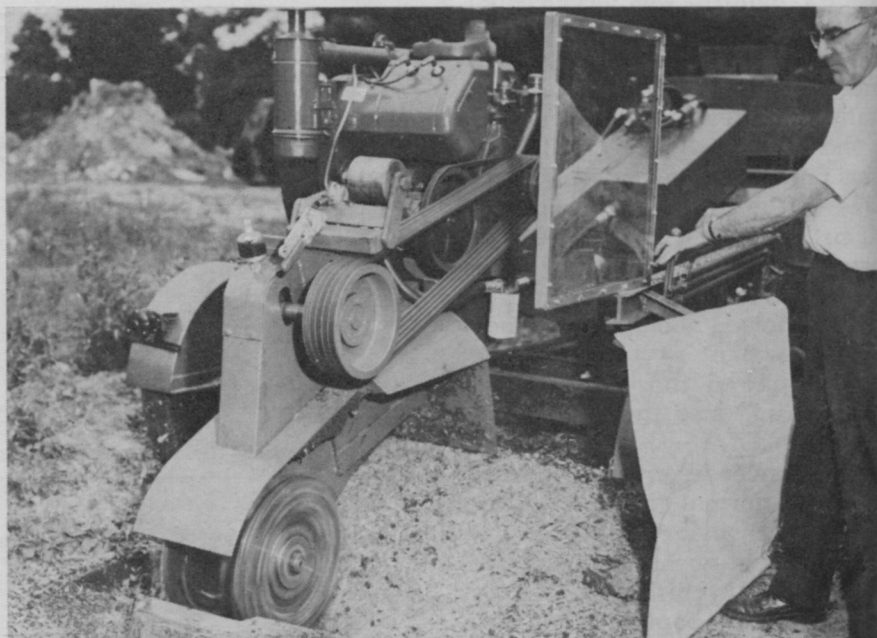
Troublesome stump in foreground was delaying landscape job until Stump-King came along. Makers of this new machine say it is ready to begin cutting as soon as it's backed up to a stump; no need to reposition unit's wheels. Blade is lever-controlled.
