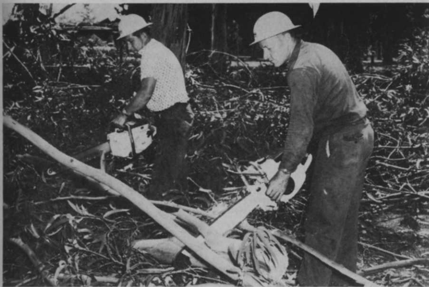
Using portable power chain saws, these men clean up the cut limbs and brush from a city street tree trimming operation. A short time before these saws were used high in the air for pruning and topping.
