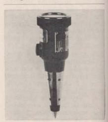
Kelway Soil Tester Model B-3 measures the acidity of soils in field or laboratory. The 3 by 7 in., 8 oz., fully guaranteed unit uses no chemicals or reagents. When inserted in soil a reading appears within a minute. Kel Instruments Co., Inc., P. O. Box 446, New Brunswick, N. J. 08903 can furnish more information.
