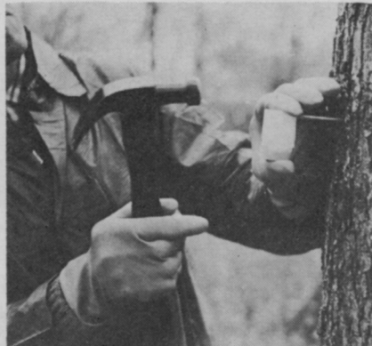
8. Gentle tapping of hammer inserts container onto aluminum tube, bottom side upward.
