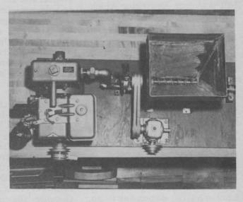
hoses are adjustable to serve a depth of 3' to 12'. By means of a V-Belt, gear reducer and clutch, the motor also drives a worm-screw feed in the bottom of a hopper. This hopper is located over the discharge line.
