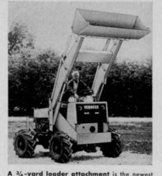
of eight quick mounting tools for Vermeer's Pow-R Ditchmaster tractor. This new loader can be mounted in a matter of minutes, the company says. The operator is seated on the front of the tractor unit for increased vision and better control. Heavy-duty 9:00x16 traction tires are driven by a 4-wheel, hydraulic, variable speed drive providing unexcelled "digging" power, it is said. Complete details are available from the company by writing Vermeer Mfg. Co., Pella, Iowa.
