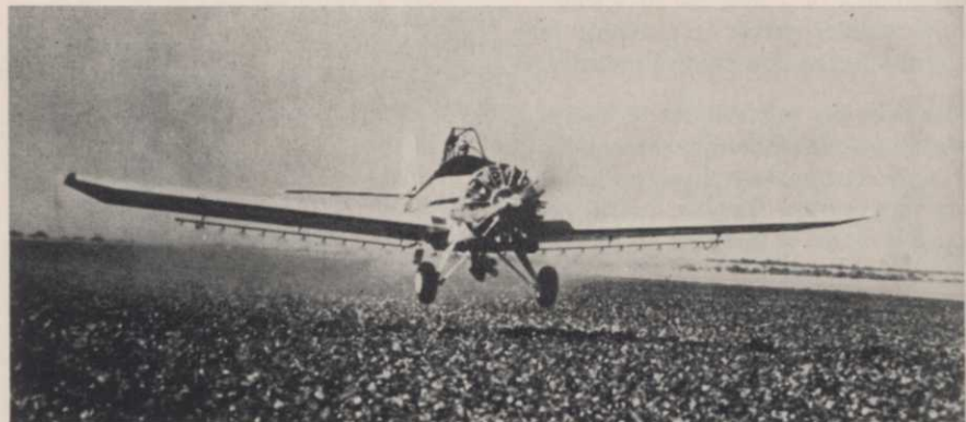
The New Snow S-2C agricultural airplane offers ag-operators and growers a wider, more uniform swath resulting from the increased span and new wingtips. Designed specifically for aerial application use, the single low wing combines the best features of downwash and vortex action to evenly distribute spray or dust, Snow reports.
