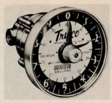
Reset dial registers to 10 gallons on the large scale of the new, stainless steel flow meter from Tryco Manufacturing Co. Inner dial will measure to 100 gallons, and 5-digit register keeps a running total of the quantity dispensed.
