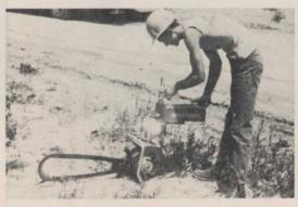
To avoid gasoline spillage this Asplundh man uses a plastic funnel which screws into the filler hole of his chain saw.
