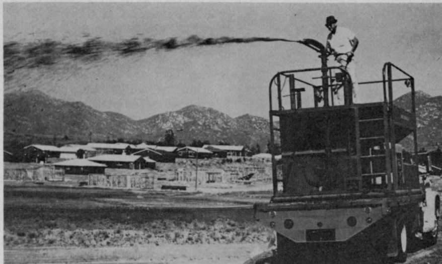
Low center of gravity and three agitators are features of the new Imperial Model Bowie Hydro-Mulcher.
