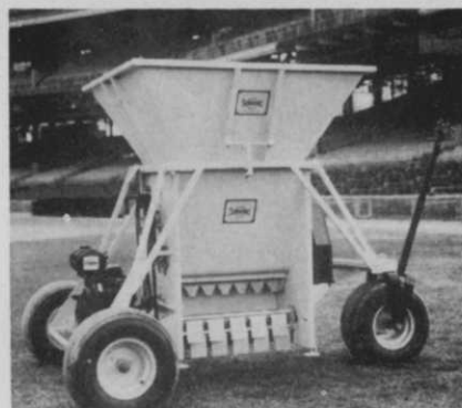
Anti-bridging agitator on the Greenskeeper, new spreader from Sunnyhill Research and Manufacturing Co., broadcasts peat moss, fertilizers, herbicides, lime, and seed, among other materials. Spreader has an independent power supply, with agitator and feeding mechanism electrically controlled by magnetic clutch.
