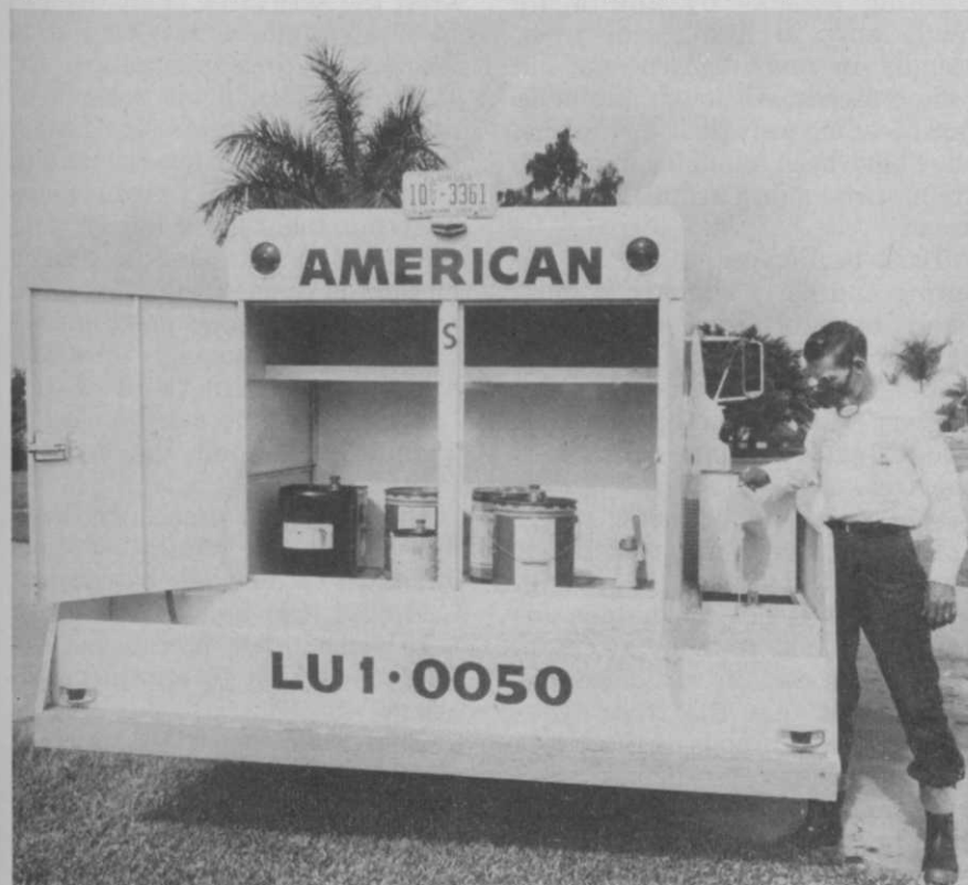
Operator can add chemical to the lower tank with ease and speed, as this sprayman demonstrates.
