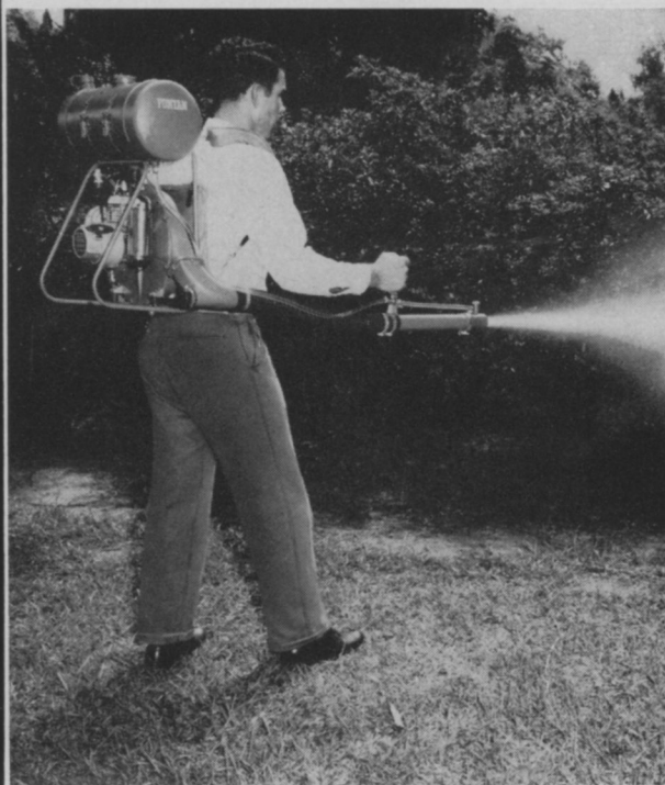
THE R.6 FONTAN FOR SMALLER JOBS WEIGHT 24 LBS.
