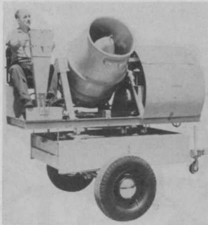
New John Bean Rotomist, with an air velocity of more than 100 mph, can rotate a complete 360° with great accuracy and balance, the manufacturer claims.
